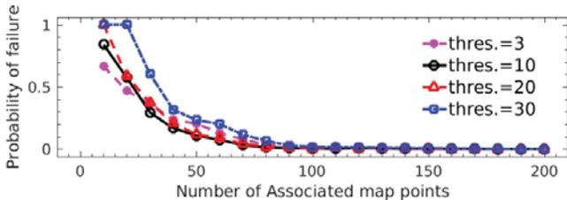
Fig. 2. The relationship between the number of observed map points and probability of tracking failure with monocular ORB SLAM on EuRoC dataset Vicon Room 1 03 and Vicon Room 2 03 sequences.
